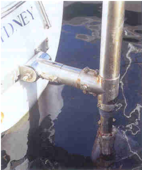
This BWS-Taurus system would be better with a V-shaped bracket at the bottom
