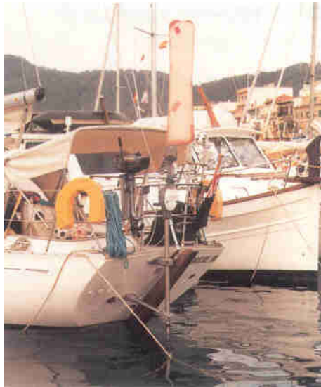
Offset mounting next to an outboard rudder. The minimum distance to the main rudder is 30cm/12in.
