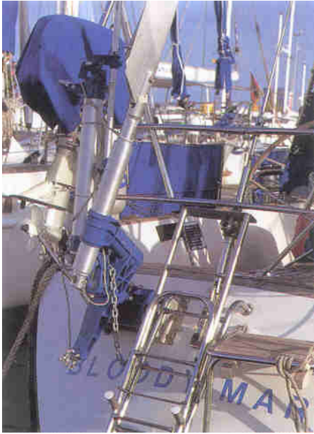
An offset mounted servo-pendulum system will not function effectively
