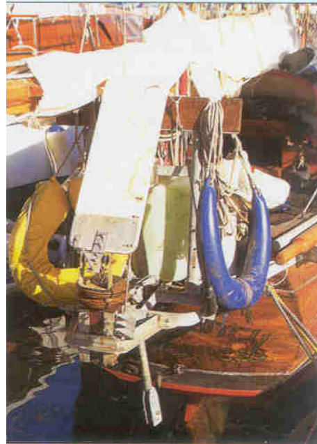
H vane only, QME windvane. This acts more as a steering aid than a full selfsteering system
