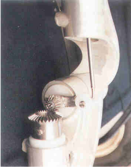
Windpilot Pacific 360 degree bevel gear linkage ratio 2:1
