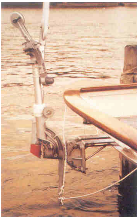
This mounting for a Windpilot Pacific on a 25 tonne gaff cutter has worked well for 12 years.
