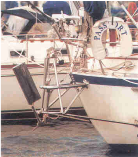
Conventional servo-pendulum systems often require the mounting components to be customised
