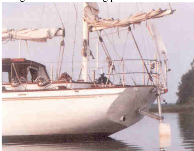
A mizzen which extends over the transom causes problems for a windvane
