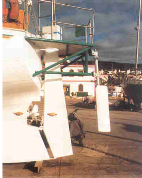
The ratio of main rudder area to auxiliary rudder area is ideally 3:1
