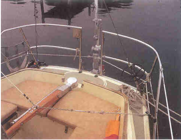
Short transmission path to the tiller with the Windpilot Pacific. The steering lines start at deck level.
