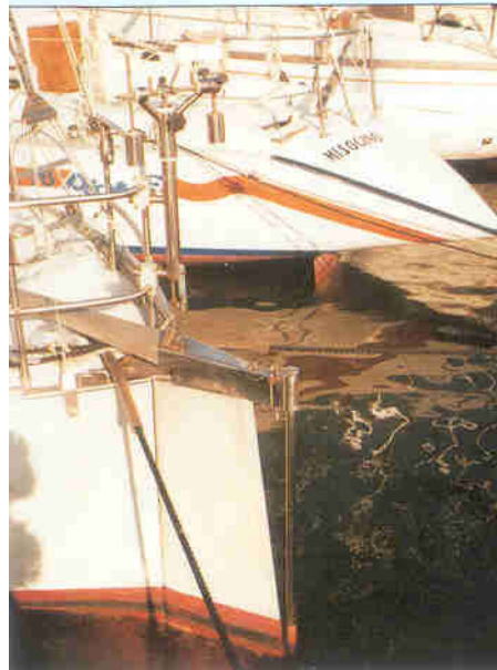
H vane trim-tab-on-main-rudder system, Windpilot Pacific custom-built for a Danish Kaskelot.
