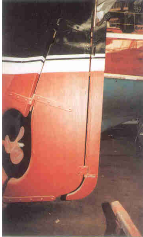
Trim tab to main rudder proportions: this system type can make reversing under power awkward.
