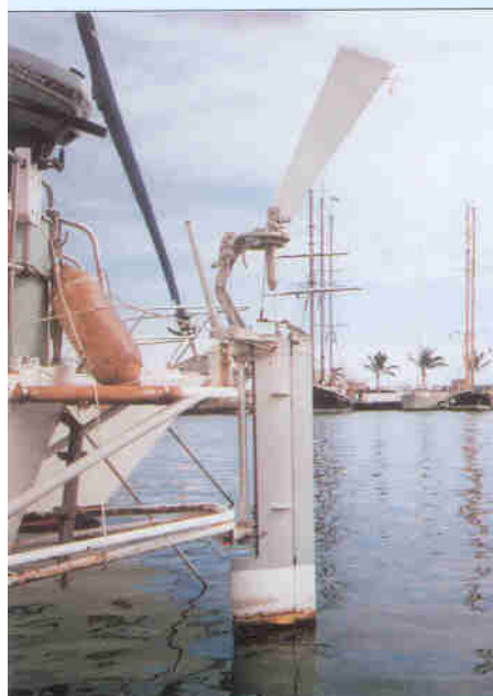
A Mustafa H vane auxiliary rudder with trim tab system – the dinsosaur among the vanes.
