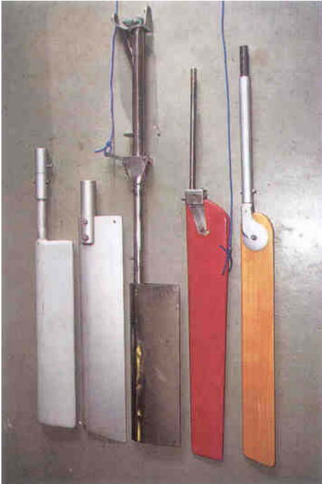
Overload protection (left to right): Aries, Sailomat, Monitor, Windpilot Pacific (old), Windpilot (new)
