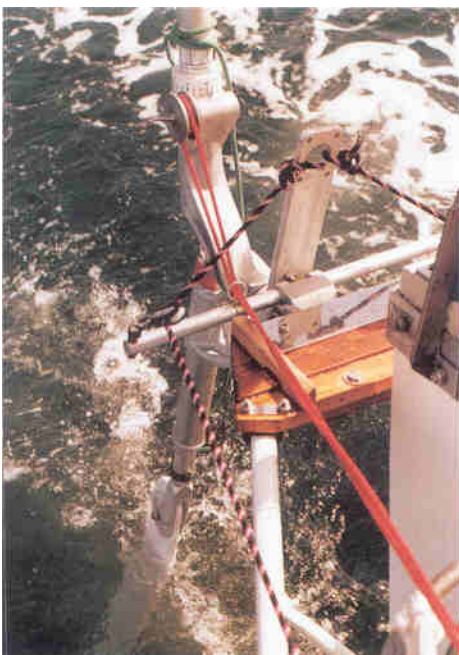
Steering line routing on a double-ender
