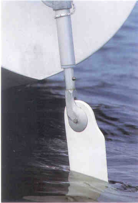
The Windpilot Pacific cuts smoothly through the water causing little drag.
