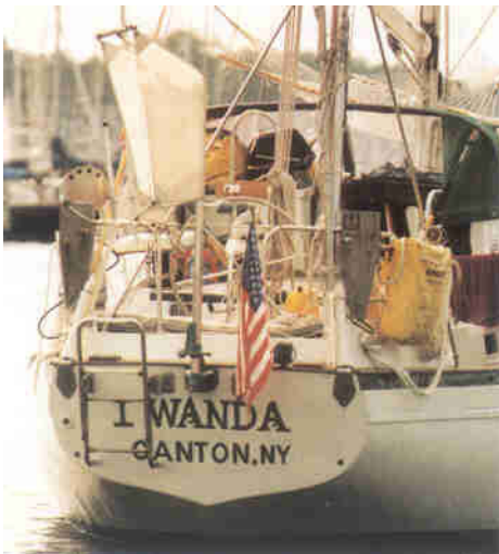
Wedge-profile V vane, Saye's Rig
