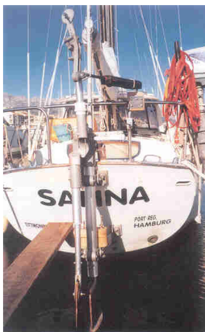
A combination of Autohelm and Windpilot Pacific Plus on a Nicholson 48.
