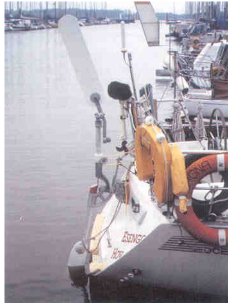
In the raised position, the pendulum rudder of the Windpilot does not stick out beyond the stern because of its angled shaft
