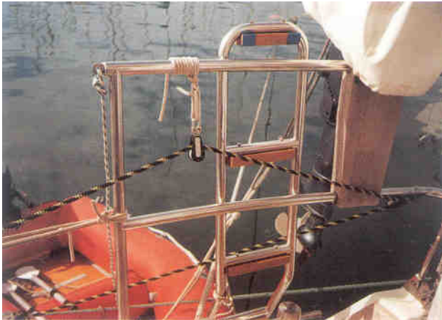
Steering lines can be tensioned easily using an additional block.
