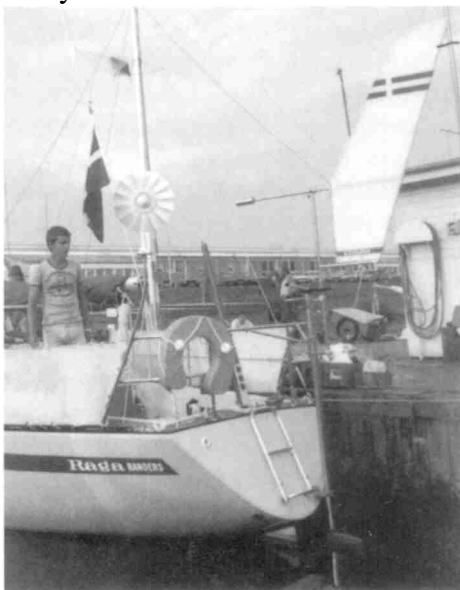
Offset mounting next to a swim ladder. The Viking ships also had their steering system positioned to one side.
