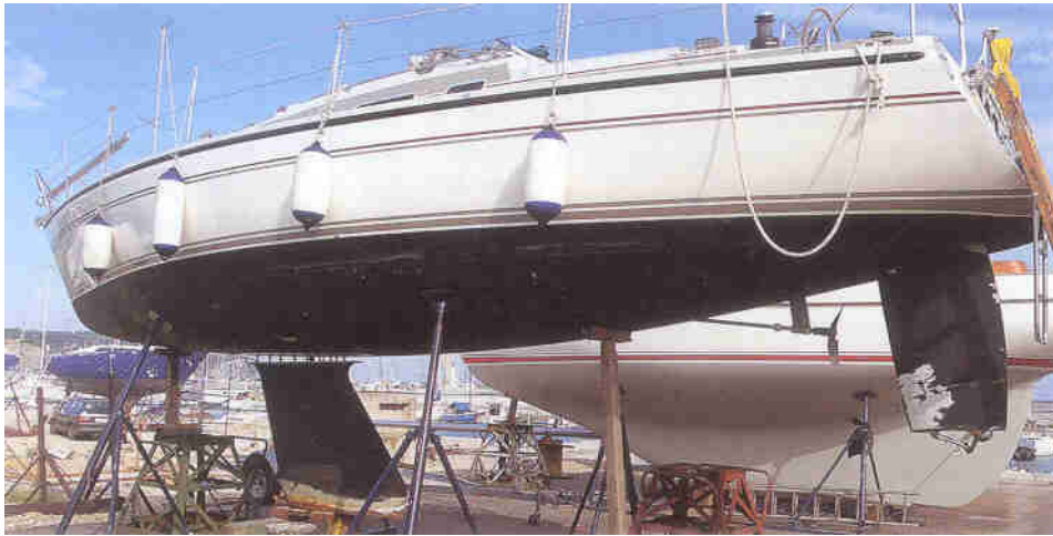
The keel and rudder of these Dehler 36 are very susceptible to damage during grounding
