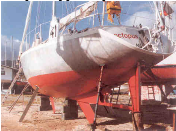
The keel and rudder of these Dehler 36 are very susceptible to damage during grounding
