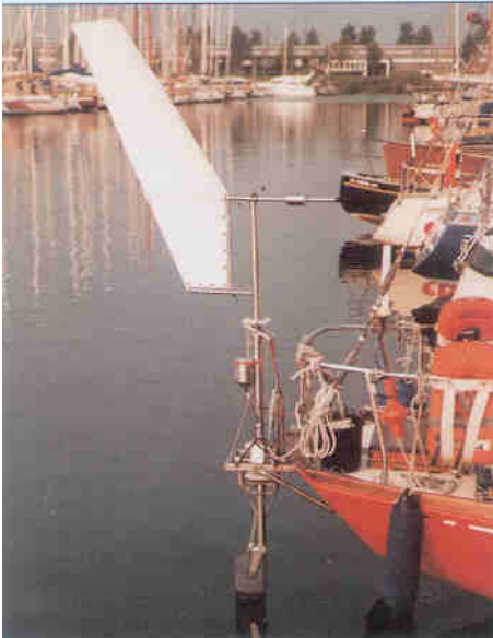
This Windpilot Pacific V vane servo-pendulum system MKI (1969), is made of stainless steel.
