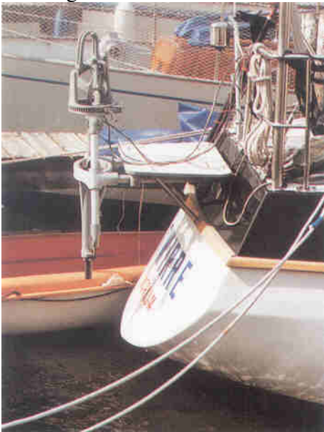
Servo-pendulum systems with a vertical pendulum arm may need extended mounting brackets on modern forward-raked transoms.
