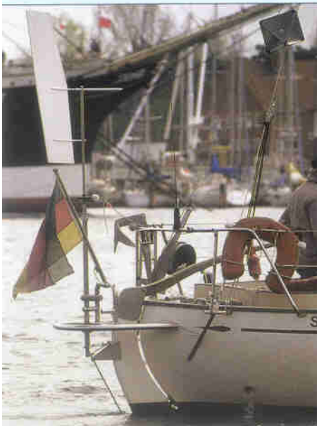
V vane trim-tab-on-main-rudder system, custom-built for a 10m/32 ft Olle Enderlein design.
