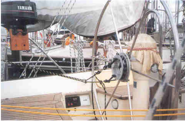
Steering lines led on one side, connection point with snap-shackles
