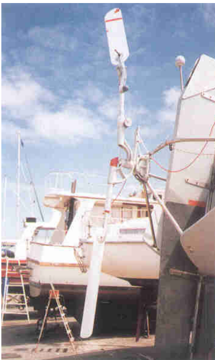
Pendulum rudder to main rudder proportions: the lever effect is the key to this system
