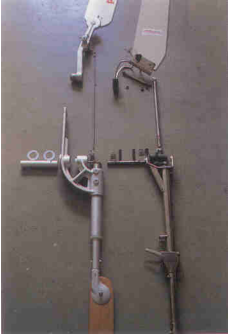
The Windpilot Pacific (left) and Monitor are identical in design, but have substantially different dimensions of pushrod, pendulum axle diameter and pendulum carriage.
