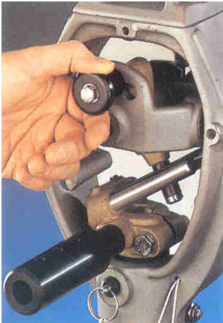
The Hydrovane linkage has step-down gearing for better damping
