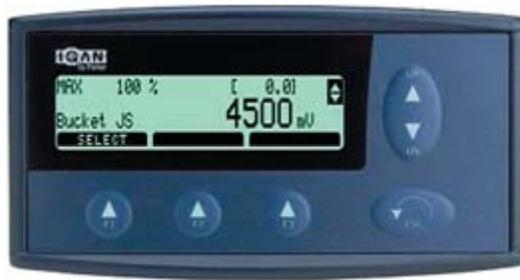
**Press the <<ESC>> Key and up arrow for the Max screen.**
