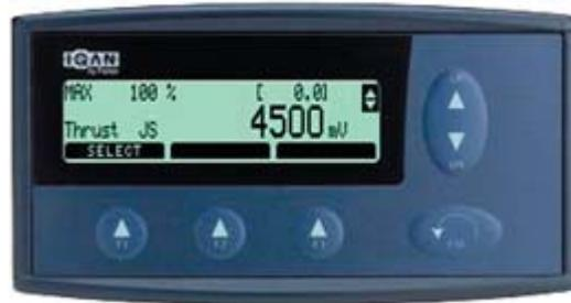
Press the F1 button to select setting the Max setting.
