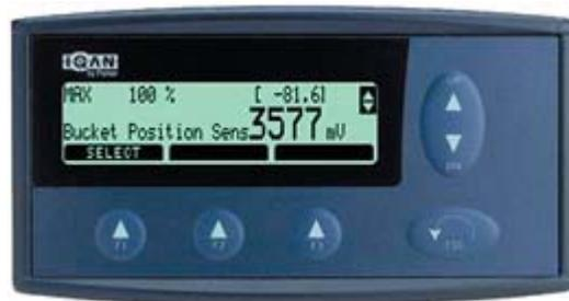
**Press the F1 button to select setting the Max settings for the bucket.**
