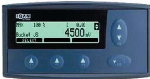
**Press the <<ESC>> Key twice to get out of the Bucket JS setting screens and press the up arrow key to move the to next screen Bucket Position.**
