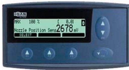
Turn the helm wheel fully to port to set the max setting.
