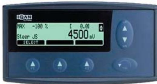
**Press the <<ESC>> Key twice to get out of the Steer setting screens and press the up arrow key to move the next screen Bucket JS**
