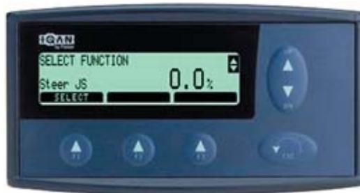
**Press the F1 button to select setting the Min/Max settings for the Jetstick steering.**
