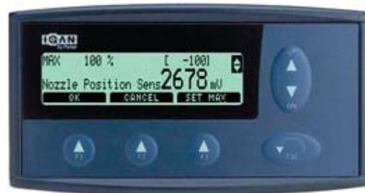
Press the F3 key to set the max setting, then the F1 OK key.
