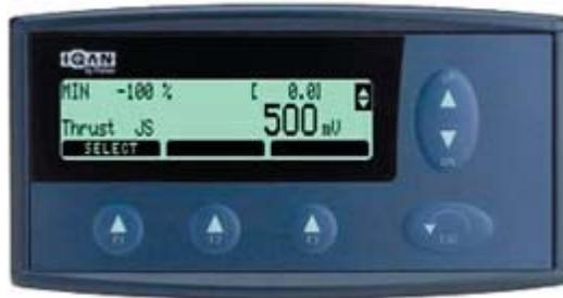
Press the <<ESC>> key and then the up arrow to continue to the Max setting screen.
