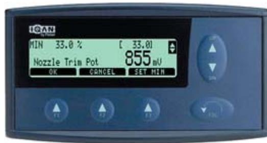
Press the F3 key to set min and then the F1 key to accept the new min valve.
