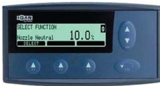
**Press the F1 button to set nozzle neutral; boat must be running and in gear.**
