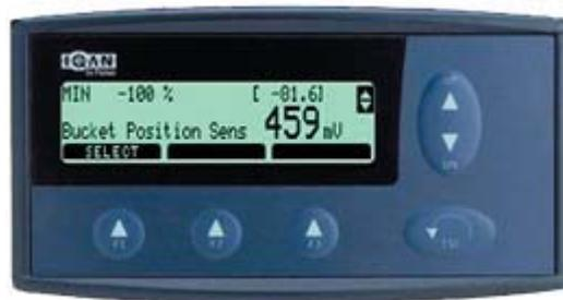
**Press the F1 button to select setting the Min settings for the Bucket Position Sensor.**
