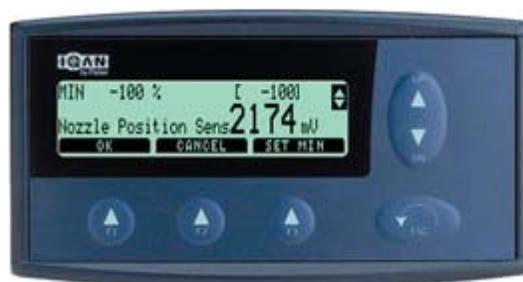
Press the F1 button to select setting the Min settings for the Nozzle. On the Mode select panel change to Helm Mode and turn the helm wheel fully to starboard.
