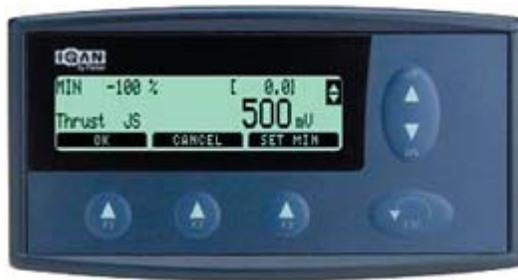
Hold the Jetstick to port and press the F3 button to set the Min. The 500 mV will change to the new Min setting or may remain the same.
