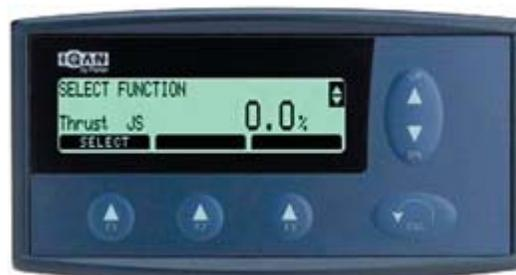
Press the F1 button to select setting the min setting.
