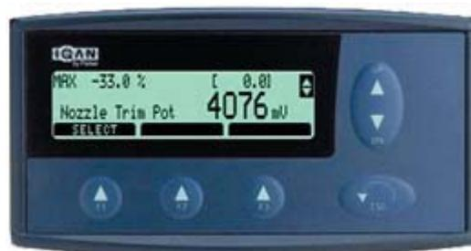
Press the F3 key to set the max then the F1 OK key.
