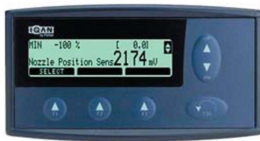
Press the <<ESC>> Key twice to get out of the Bucket setting screens and press the up arrow key to move the to next screen Nozzle Position.
