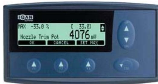
Turn the trim pot fully starboard and press the F1 key to select
