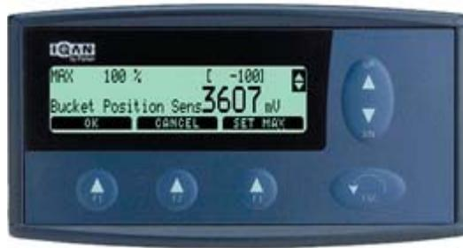
With the bucket fully Up press the F3 button and then the F1 OK button to record the new max setting.
