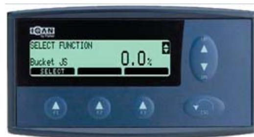
**Press the F1 button to select setting the Min/Max settings for the Bucket JS.**
