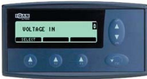
Press the F1 button to select the first screen, Thruster Jetstick.
