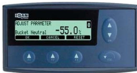
Using the up-down arrow key, adjust Bucket Neutral in the desired direction. More negative lowers the bucket and less negative raises the bucket. This number will never be a positive number. Once desired neutral is obtained press the F1 or button.
