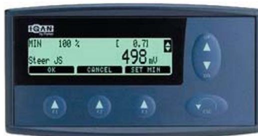
**Press the <<ESC>> Key and then the up arrow to get to the max screen and select by pressing the F1 Key**
