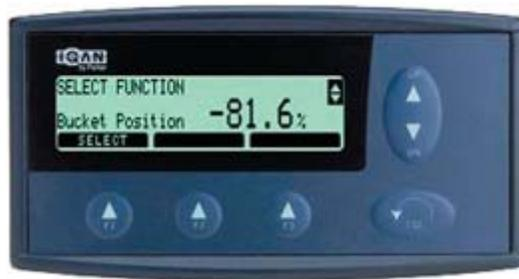
It is important that the bucket position transducer be mounted so that the down reading is as close to 500 mV as possible.
