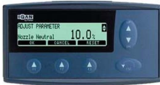
**Nozzle Neutral is best set with the boat off the dock, pointed into the wind with RPM about 1500. Watch for a steering bias in either direction and change the value accordingly. This number can be a positive (port) or a negative (starboard) number.**
