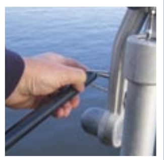
The extendable tiller arm is secured to the Windpilot
