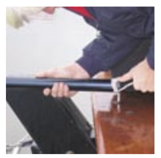
The tiller pilot fits into a hole drilled into the wooden capping
