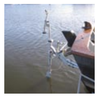
The pendulum servo gear with the paddle in the water
